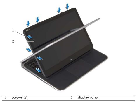
4 Starting from the corners, gently pry the display back-cover from the display panel.
